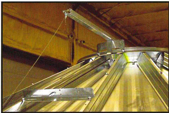
The ground control Remote Opener is standard on all hopper bins.
